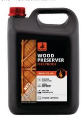
A water-soluble ready to use preserver based on modified, inorganic potassium compounds that protects wood against fire. Does not corrode steel. Lowers the freezing point of the working solution to -7°C. Properly secured wood, in accordance with the National Technical Assessment of ITB, is a non-combustible material.
